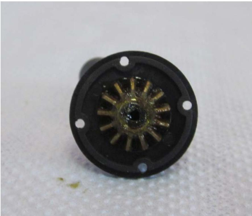
Grease the insides of the differential with suitable grease.
