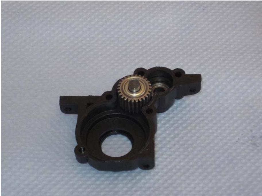
Pull the spacer and the gear wheel from the shaft.
