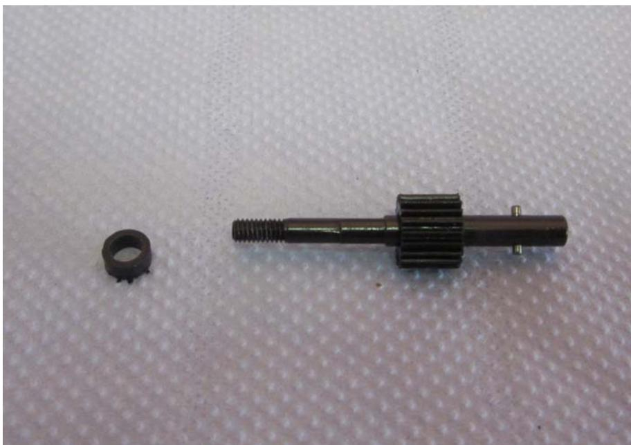
Slide the metal gear wheel onto the shaft and fix the metal gear wheel on the carrier.
