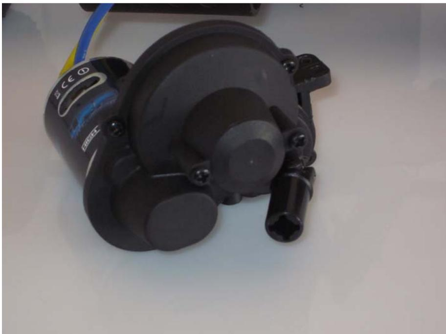
Insert the gear unit into the car now. In doing so, put the drive shafts into the differential outdrives.
