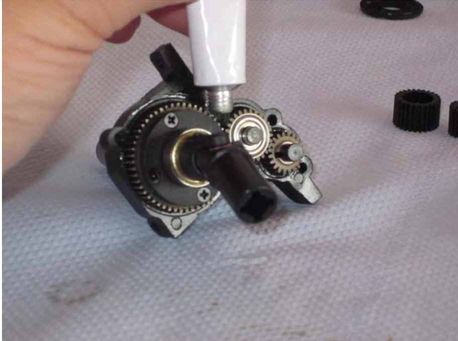
Put the two parts of the gear housing together and insert the marked screw (see next page).
