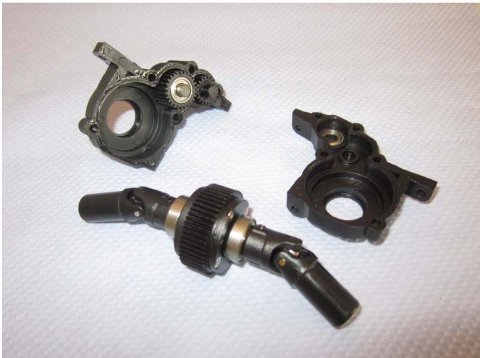
Take out the middle gear wheel and the slipper shaft now.
