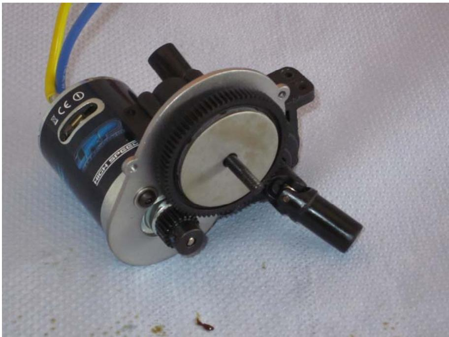
Assemble the washer, rebound spring and nut of the slipper. Setup the slipper as described in the manual of your S10 Twister car. **Please check the pinion clearance by all means.**
