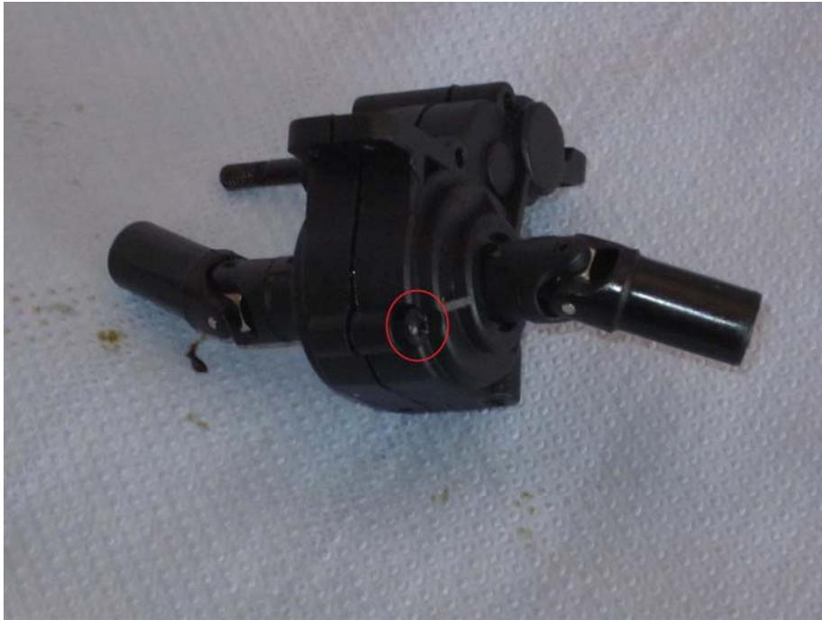
Position the motor mount on the gear housing and fix it with the four screws. Tighten also the screw marked on above image.
