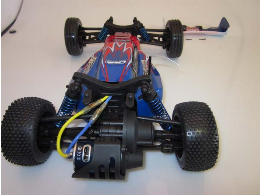
Disconnect the motor cables and loose both of the marked screws.
