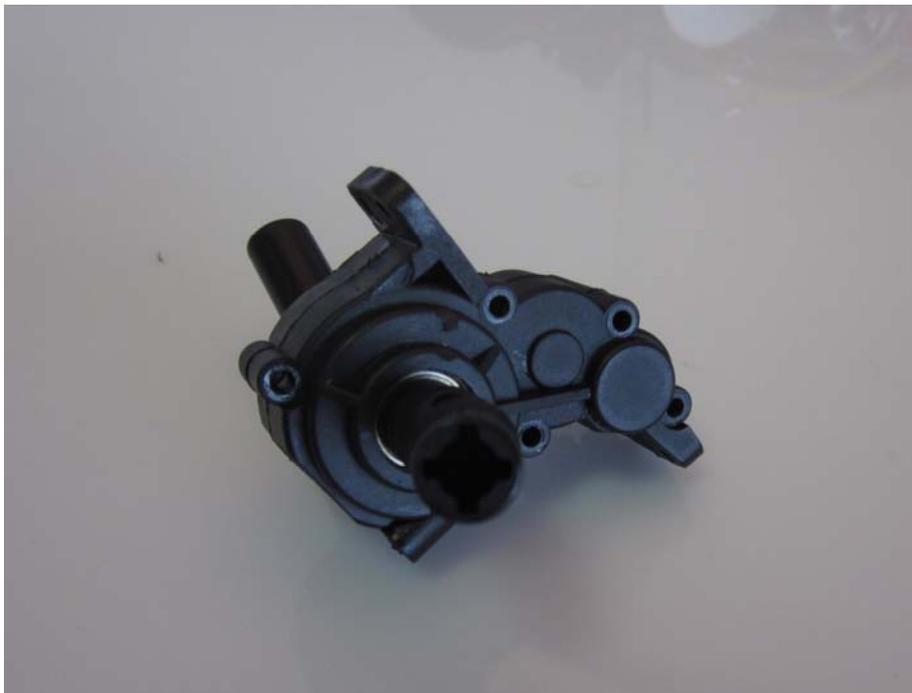
As the gear parts are greased, please make sure you use some kind of underlay or pit towel from now on! Open the gear box as shown on the image.
