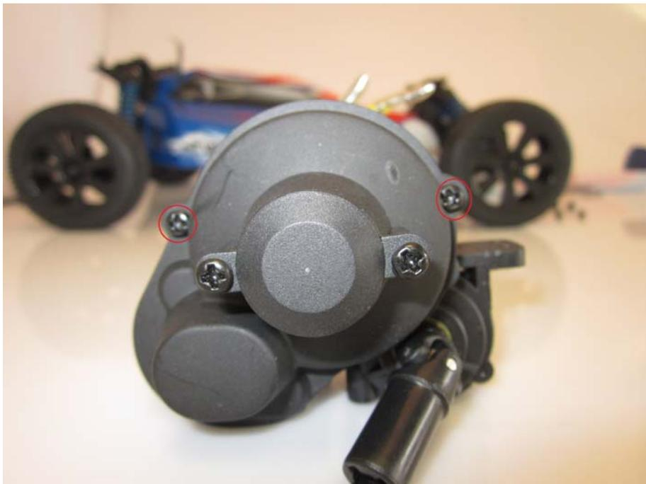
Loose the nut of the slipper and remove all of the components from the slipper shaft.
