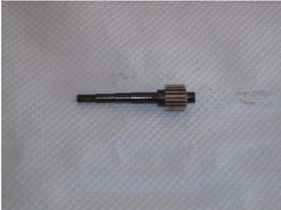
Insert the slipper shaft with the metal gear wheel into the gear housing.
