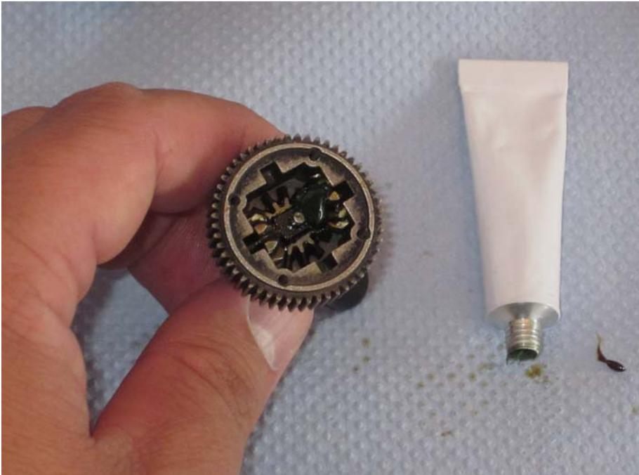
Shut the differential with the four screws included in the metal gear set.
