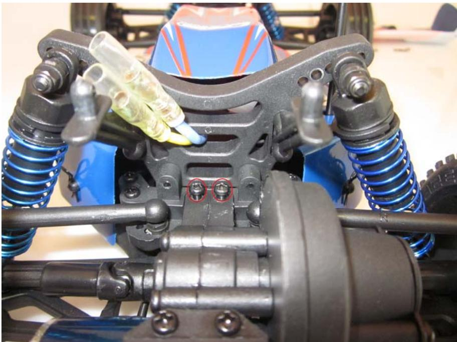
Loose both of the screws of the motor protection.
