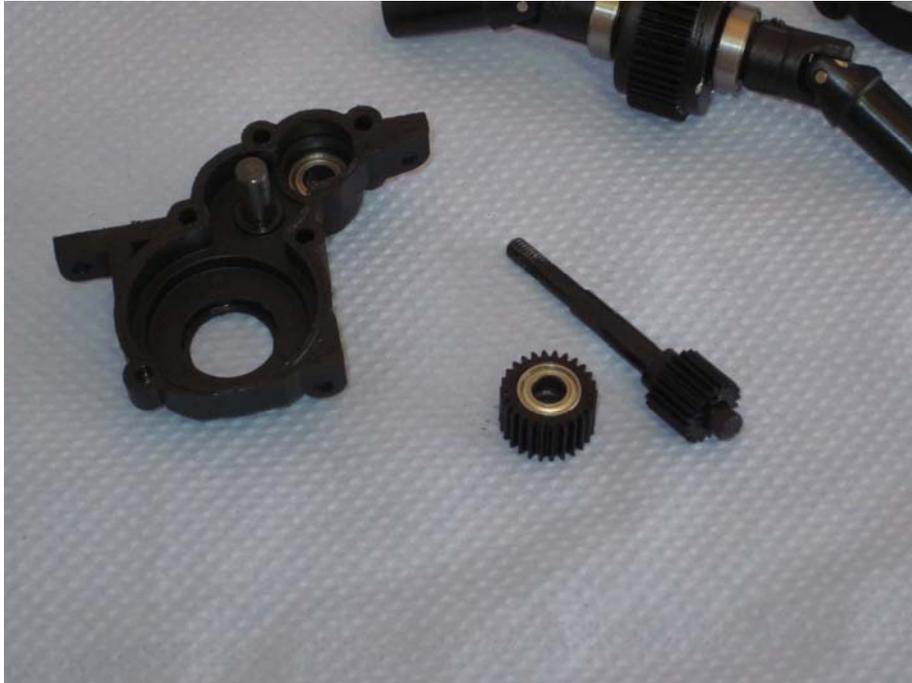
Then, remove the ball bearings from the middle gear wheel.
