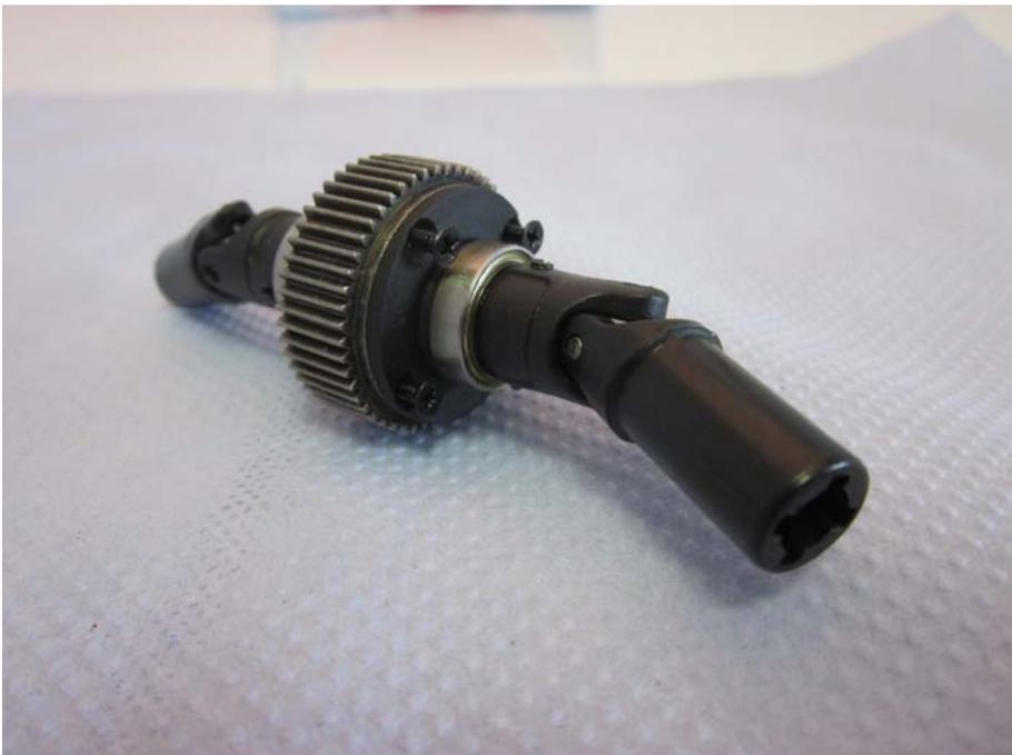
Insert the differential into the gear housing and grease the gear wheels.
