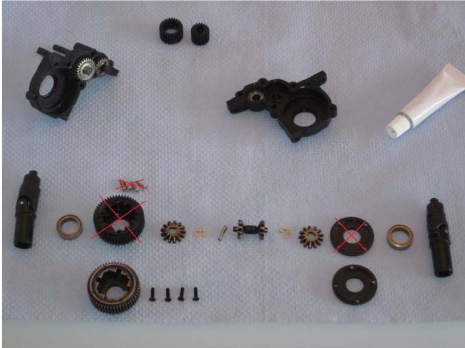
Reassemble the two sides of the differential in reverse order.
