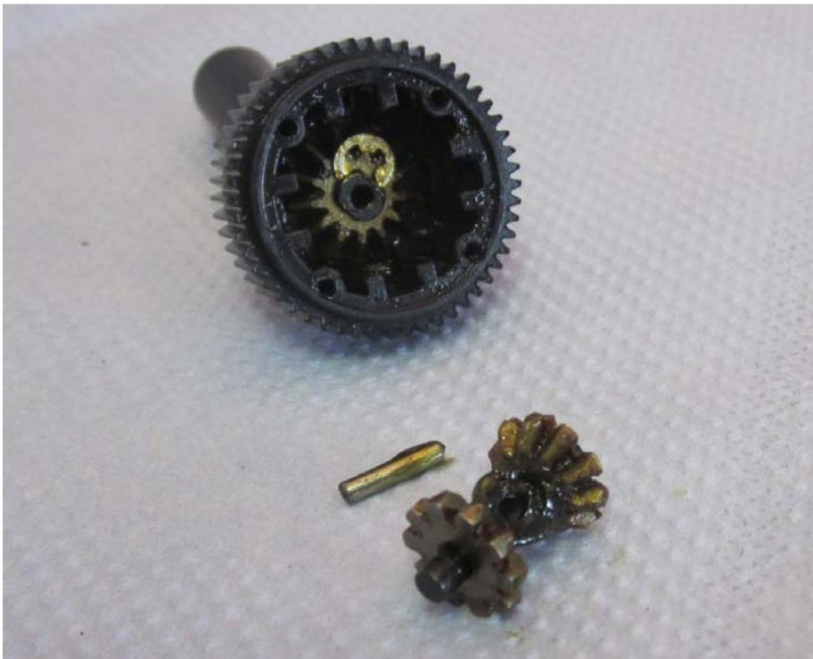
Clean all gear wheels. The crossed out parts have to be replaced by the new components that are shown below.
