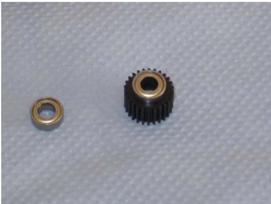
Insert the ball bearings into the metal gear wheel. Build the metal gear wheel into the gear housing.
