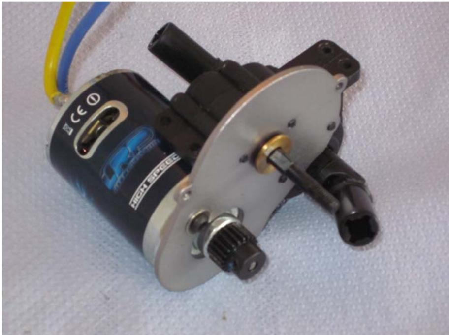
Then, assemble the pressing disks, slipper disks and main gear as shown on the images. Please mind the recesses of the slipper disks. These have to match the main gear.
