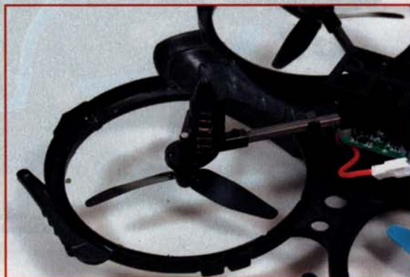
There is a little motor on each corner that provides plenty of power. The props are protected by a foam outer frame
