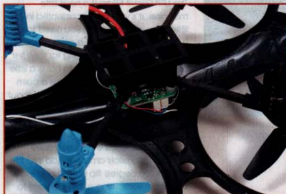
The LiPo battery pack sits in a cradle underneath the model for the best centre of gravity. The six-axis gyro and receiver sit above it
