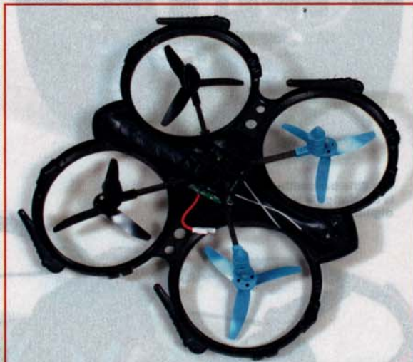
Here you can see the simple structure surrounded by a foam frame. The quad uses blue props on the front and black on the rear
