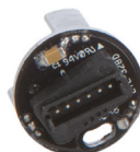
Left: The X20's rotor is etched with its size for easy tech inspection.
