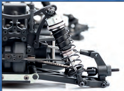
Right-left threaded rods are just as much a part of the package as the "big bore" oil shock absorbers on both axes
