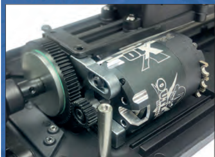
Slipper clutch and aluminum motor mount.
