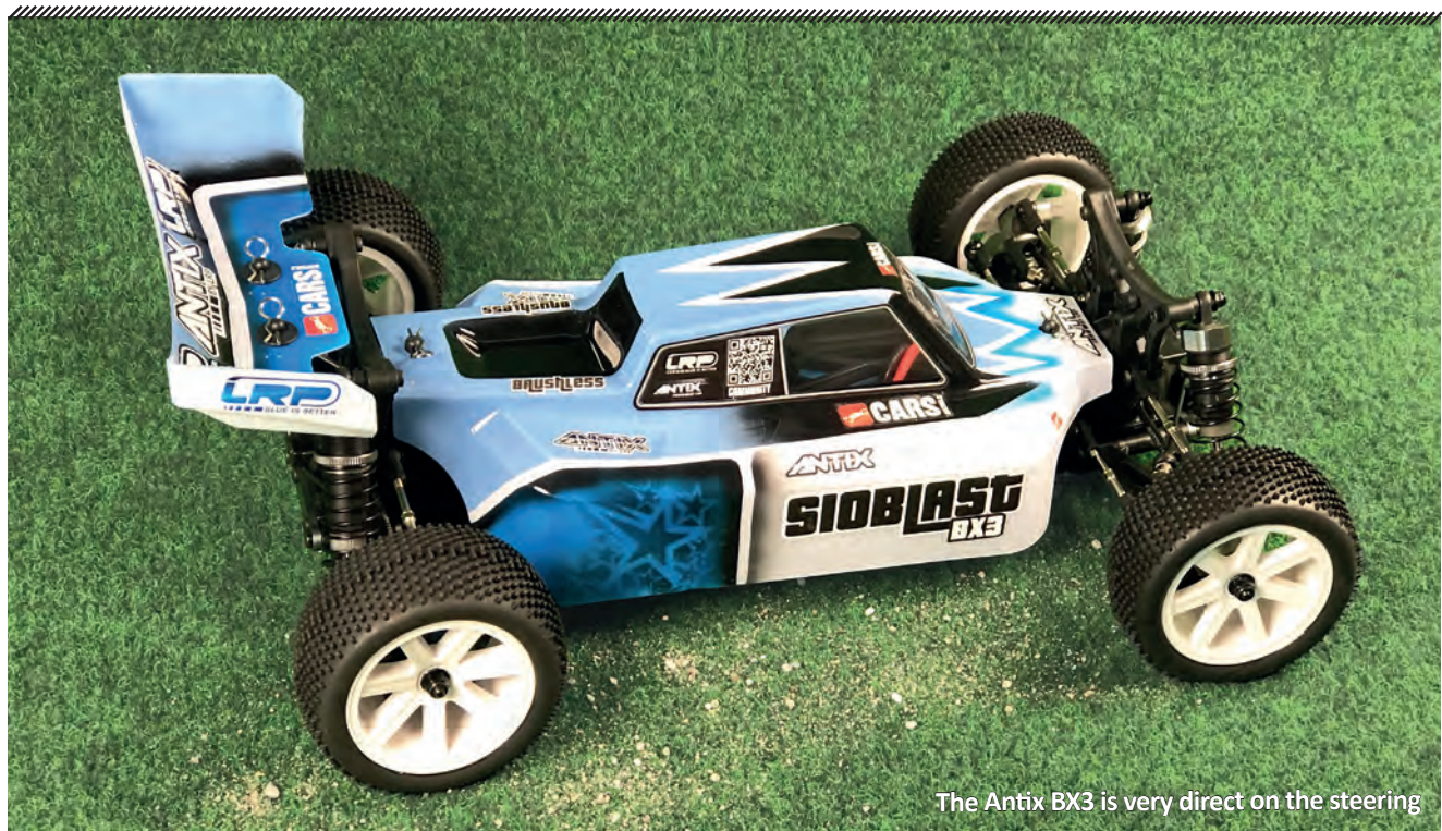
Right-left threaded rods are just as much a part of the package as the "big bore" oil shock absorbers on both axes
