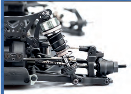
Right-left threaded rods are just as much a part of the package as the "big bore" oil shock absorbers on both axes
