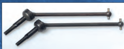
The front wheels are driven by CVD shafts. Bone shafts are used at the rear.
