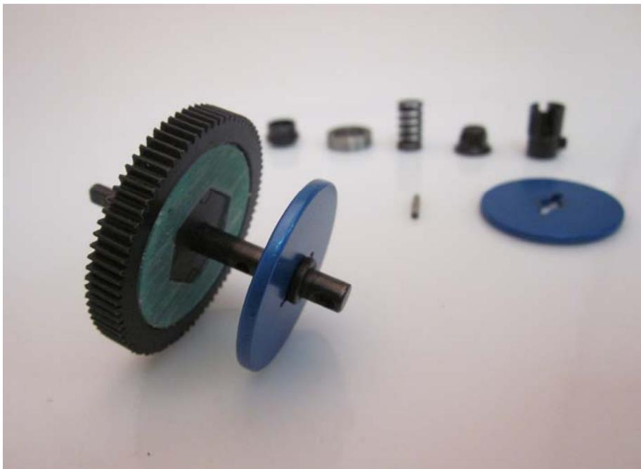
Remove the slipper pads from the main gear.
