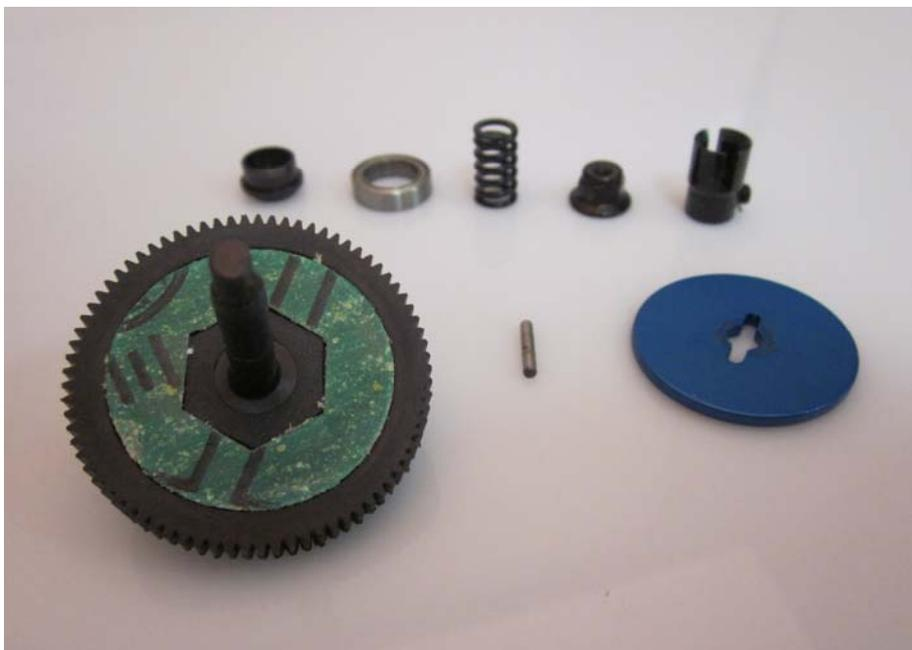
Insert the adapter pin into the shaft. Then, mount the metal disc.
