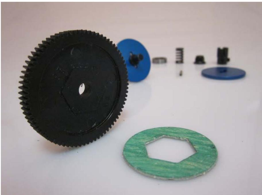
Mount the main gear onto the slipper shaft.
