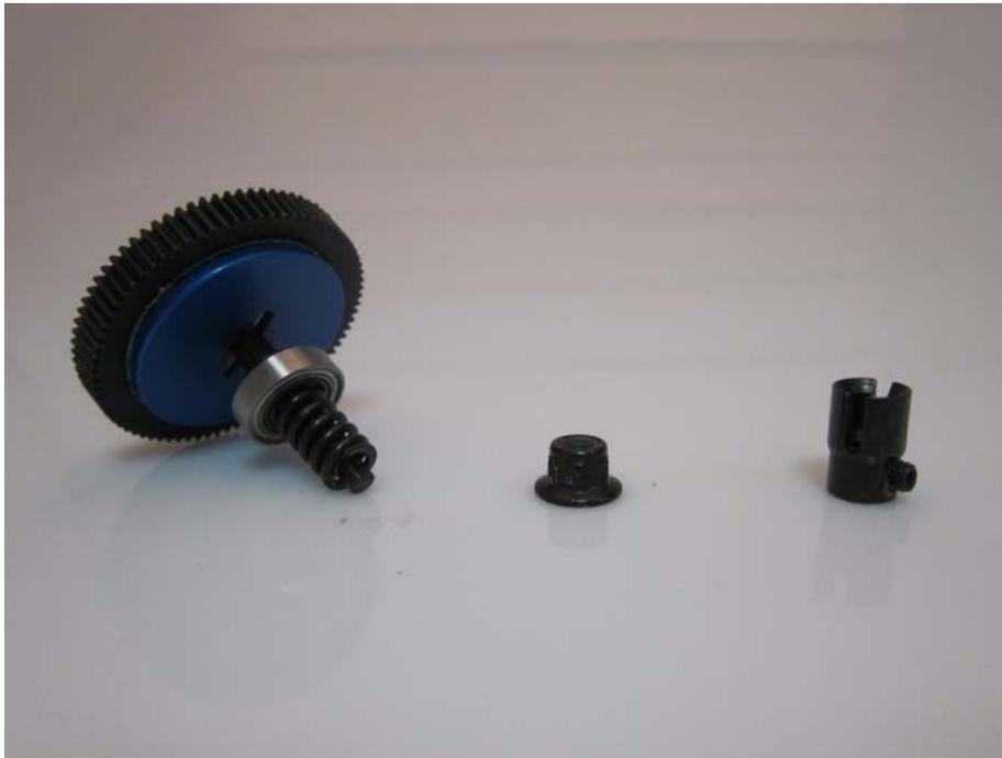
Remove the spring, the ball bearing and the bushing of the spring.
