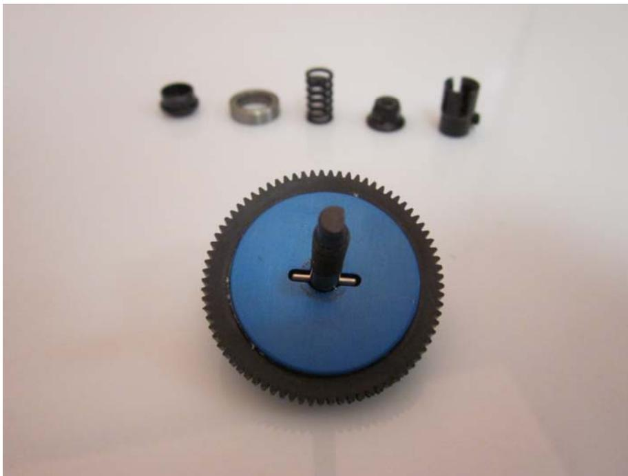
Remove the metal disc from the shaft. Please make sure the adapter pin doesn't get lost.
