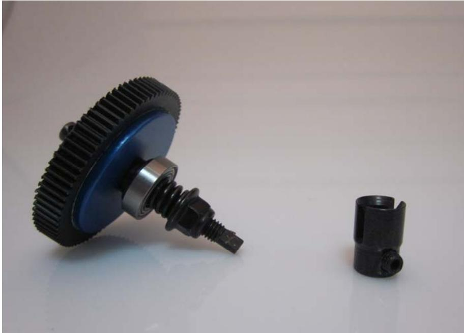
In a final step, mount the dogbone-outdrive for the centre drive shaft. Please make sure the locking screw is placed on the flat portion of the shaft. Insert the locking screw with screw locking varnish.
