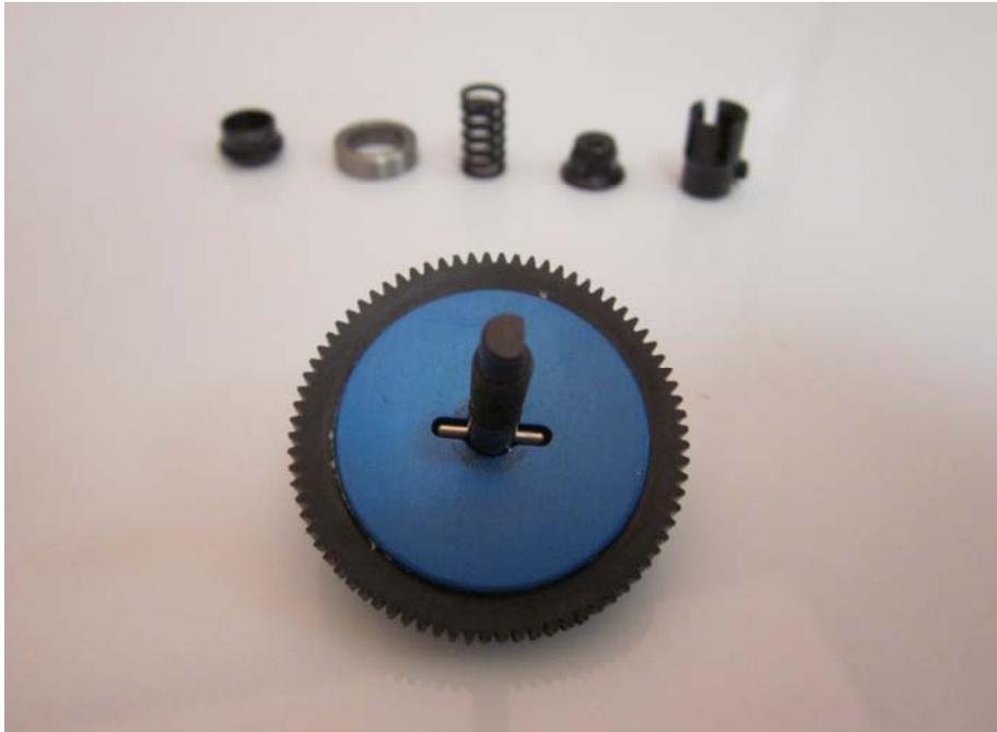
Fit the bushing onto the shaft. Then, fit the ball bearing and the spring onto the shaft. Stretch the spring with the self-locking nut. Setup the slipper as described on page 1.
