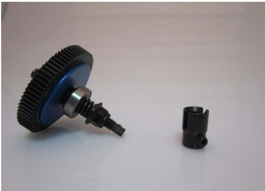
Slack off the rebound spring by loosening the self-locking nut of the slipper.
