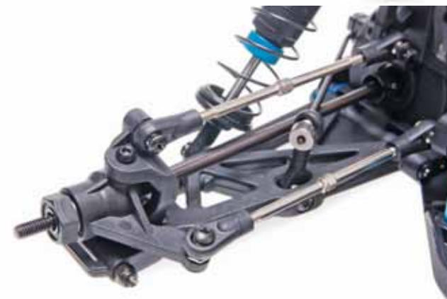
Above: C-hubs, H-arms, steering knuckles, just proven RC design here. Note the nutted hinge pins—anyone remember e-clips? No? Good. Right: The plastic-body shocks are well built and classed up with aluminum caps and preload collars.
