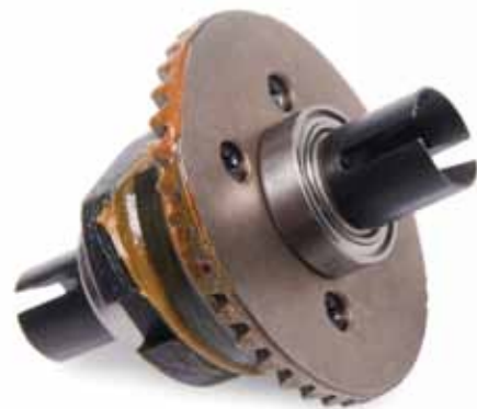
Sealed bevel-gear diffs are standard.
