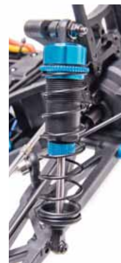
Above: C-hubs, H-arms, steering knuckles, just proven RC design here. Note the nutted hinge pins—anyone remember e-clips? No? Good. Right: The plastic-body shocks are well built and classed up with aluminum caps and preload collars.
