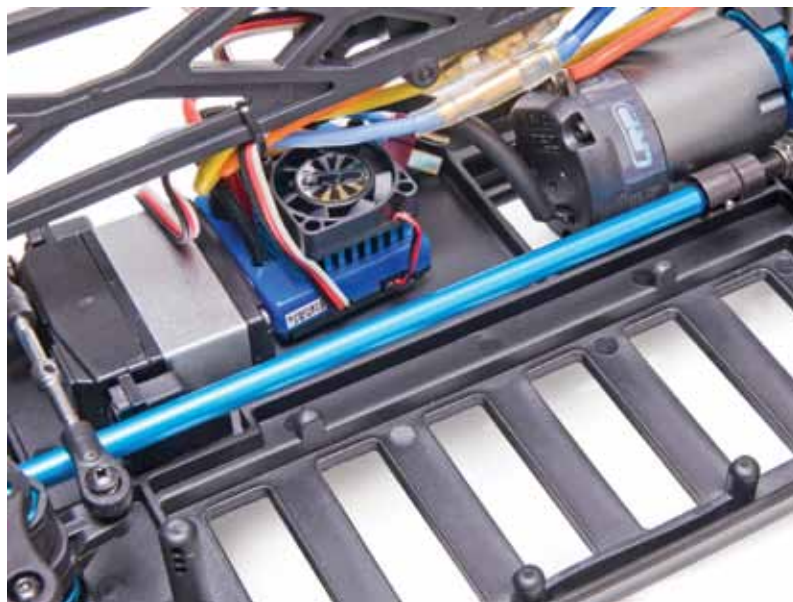
Left: The Blast's blue-anodized slipper clutch and motor mount look like they belong on a more expensive truck. Below: Many RTRs sneak in a plastic shaft, but the Blast has an aluminum shaft for high power capability.
