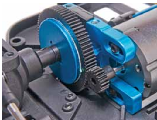
Left: The Blast's blue-anodized slipper clutch and motor mount look like they belong on a more expensive truck. Below: Many RTRs sneak in a plastic shaft, but the Blast has an aluminum shaft for high power capability.
