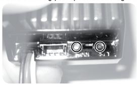
**Step9:** close your speed-control again by attaching the new lower case (as supplied), you recognise the new type by the extra pocket in the middle.
