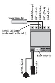
**Receiver Connecting Wire:** The SXX Version 2 is equipped with an LRP Multicon receiver wire. As supplied, it will easily fit in all ordinary receivers. Make sure you connect it to receiver with correct polarity and use chan nel 2.
