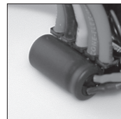
Mount the power-capacitor in a position where it is protected in the event of a crash. The best place is right next to the speed-control (see picture). Secure it with doubled-sided tape.
