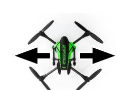
4. To fly forwards or backwards -> Push your RIGHT control stick to the front or back. The further you push the stick, the faster the Gravit will fly forwards/backwards.
