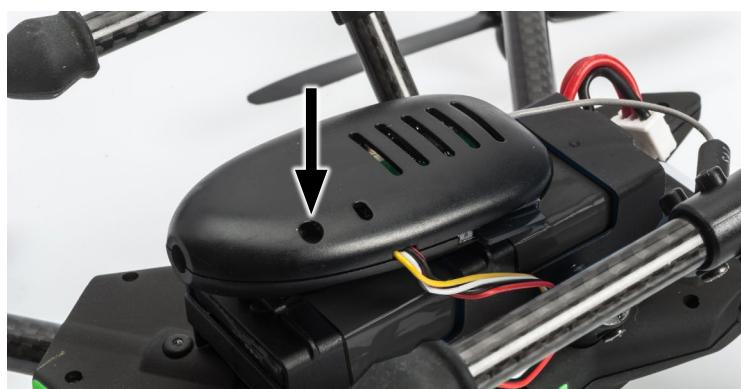
Ex works, the camera is set to transmit on CH1. If you take a small tool and press the camera button once, you will hear/feel a click and the camera switches to the next channel, which is CH2. Every further press on the little button will make the camera switch to the next higher channel.
