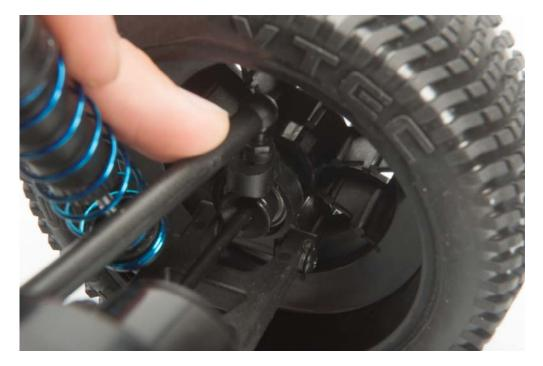
Make sure the suspension moves smoothly and the wheel rotates freely. **Repeat on the other side of the vehicle**.
