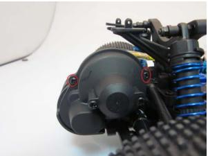
Remove the gear cover and loose one of the Phillips screws of the motor. Please take care not to lose the washer. Take the washer and put it onto the button head hex screw.
