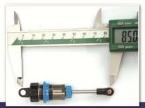
DISASSEMBLE THE SHOCK, REMOVE THE SPRING AND MEASURE THE FOLLOWING PARAMETERS (AS SHOWN ON THE IMAGES ON THE RIGHT): OVERALL LENGTH WHEN SHOCK IS COMPLETELY PULLED OUT AND WHEN SHOCK IS COMPLETELY RETRACTED; MEASURE ALSO THE WIDTH.
