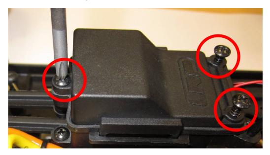
Loosen the two screws on the left and right side of the receiver box.
