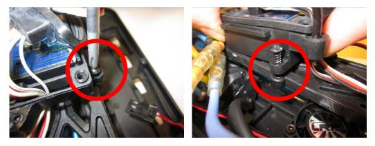
Thread the cooling fan cable first through the opening on the front side of the bottom of the receiver box and then through the rubber seal. Loosen the rubber seal from the bottom of the box beforehand.
