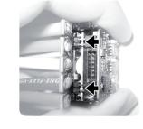
Step8: doublecheck both plastic button activators are still in place before closing your speed-control again!
