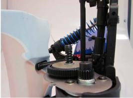
Remove the spring from the shaft. Afterwards, remove also the washer, the metal disc and the main gear with slipper pad from the shaft.
