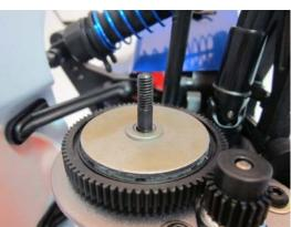
Now, fit the slipper spring and the nut onto the shaft. Stretch the spring with the self-locking nut. Setup the slipper as described above. Mount the gear cover as well as the wheel and the body shell. You're done!
