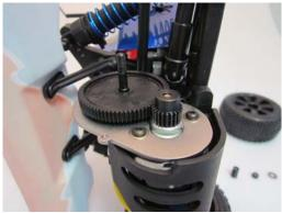
Place the second slipper pad onto the main gear and mind the flat portions. Mount the big slipper disc and subsequently the washer onto the shaft.
