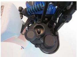
The slipper can be adjusted with a 7mm socket wrench (LRP #65721). Please close the mounting flap when you finished the setup.
