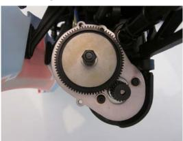
Slack the rebound spring by loosing the nut of the slipper.
