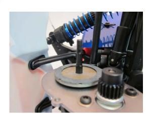
As a next step, please remove the second slipper pad as well as the lower metal disc. Then, fit the new slipper pad onto the main gear. Please mind the notches to fix the slipper discs. Otherwise, the slipper won't work flawlessly.
