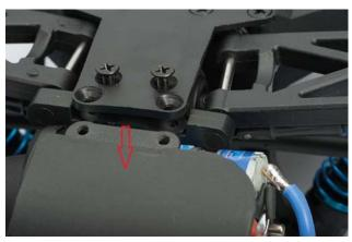
Detach the suspension arm holder backwards. Make sure that the guiding bushings remain on the suspension arm pins.
