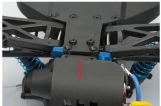
Insert and tighten the screws of the rear suspension arm holder. Please keep on making sure the plastics spacer is placed correctly. You can also use a small screw driver to keep it fixed. Tighten the screws of the gear housing now.
