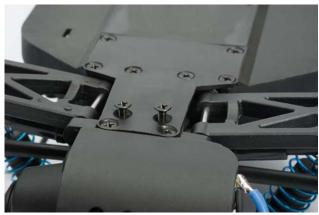
Loose and remove the two screws of the rear suspension arm mounting. Detach the motor protection cover backwards. *Attention:* there's a plastics spacer between the chassis plate and the rear suspension arm holder.
