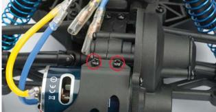
Connect the motor cables. Yellow to yellow and blue to blue. In a final step, mount the wing again. Take care of the position of the washers.
