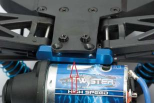
Insert the plastics spacer into the aluminium suspension arm holder as shown on the image. Mount the motor protection cover between the chassis plate and the plastics spacer. Make sure the plastics spacer does not slip out of position.
