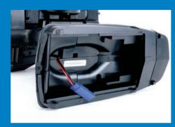
A flat LiPo falls into place in the base that means the radio is nicely balanced in use
