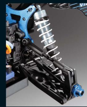
from the center diff to the front and back end. Power is sent to the front wheels by way of CVD style driveshafts while the back end uses dog bones.
