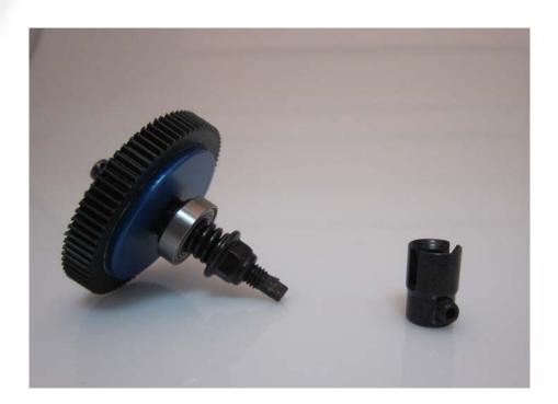
In a final step, mount the dogbone-outdrive for the centre drive shaft. Please make sure the locking screw is placed on the flat portion of the shaft. Insert the locking screw with screw locking varnish.
