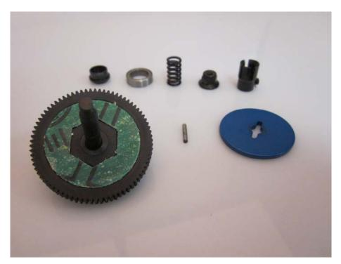
Remove the main gear from the slipper shaft.
