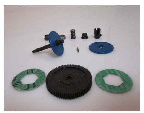
Take the new slipper pads and place them onto the main gear. Please make sure the slipper pads are correctly placed on the hexagon of the main gear. The slipper won't work otherwise.
