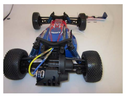
Disconnect the motor cables and loose both of the marked screws.
