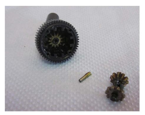
Loose the E-clip of the bevel gear with a screwdriver or pliers.
