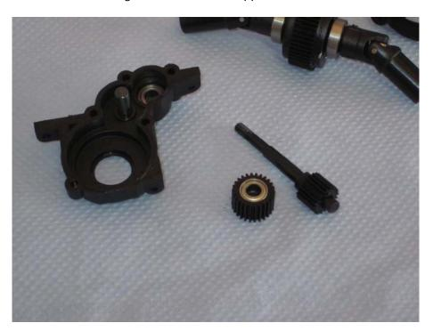
Then, remove the ball bearings from the middle gear wheel.
