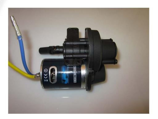
Loose both of the screws of the gear cover and remove it.
