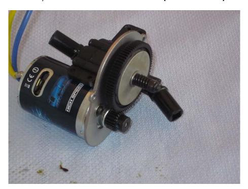
Fit and tighten the gear cover.
