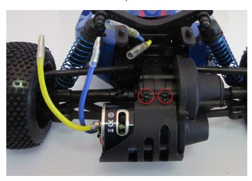
Then, loose the two lower screws of the gear box.
