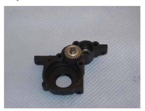
Pull the spacer and the gear wheel from the shaft.
