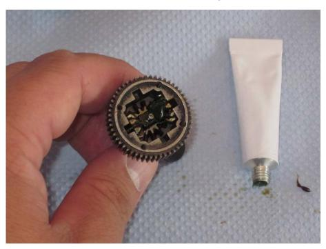
Shut the differential with the four screws included in the metal gear set. **ATTENTION:** Please do **not** use the screws of the plastic differential. In this case, you would destroy the metal differential.
