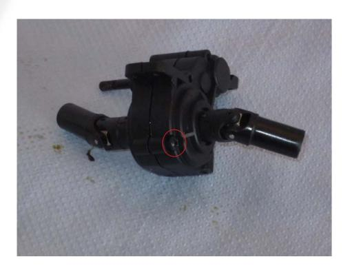
Position the motor mount on the gear housing and fix it with the four screws. Tighten also the screw marked on above image.
