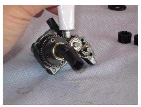
Put the two parts of the gear housing together and insert the marked screw (see next page).
