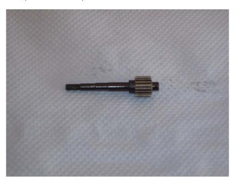
Insert the slipper shaft with the metal gear wheel into the gear housing.
