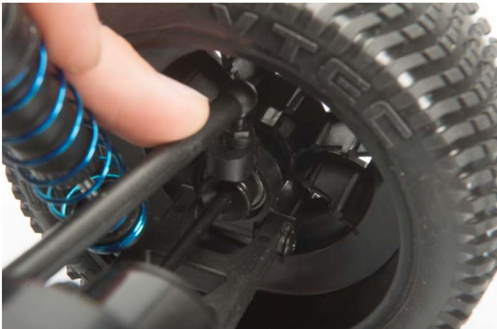
Make sure the suspension moves smoothly and the wheel rotates freely.
