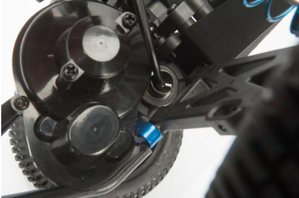
Insert the other end of the dogbone into the outer outdrive, stand the wheel up straight and press the turnbuckle back onto the ball head.
