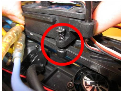
Thread the cooling fan cable first through the opening on the front side of the bottom of the receiver box and then through the rubber seal. Loosen the rubber seal from the bottom of the box beforehand.
