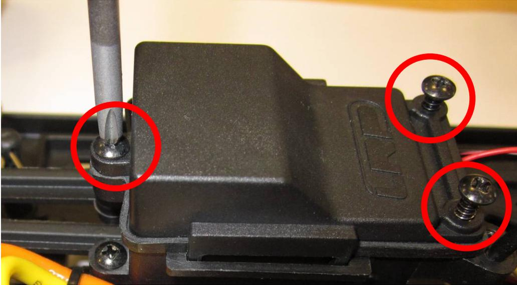
Loosen the two screws on the left and right side of the receiver box.
