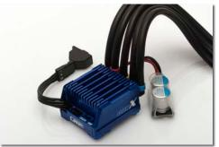
Finally, rounded off with pre-soldered all black 12AWG power wires, short receiver lead and astonishing new dark blue full aluminium case with aluminium
