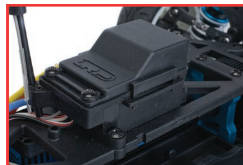
The receiver sits in its own moulded box located on the moulded top deck
