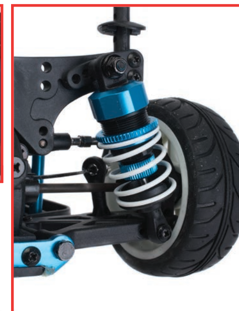
The white springs are towards the soft end of the spectrum
