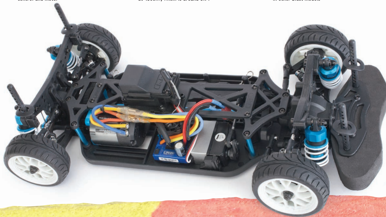
Bullet connectors are used between the speed control and motor
