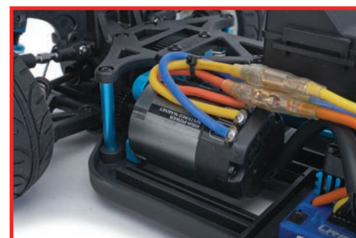
LRP's K7 Vector brushless sensor motor is rated at 4300Kv, which is around 8.7T
