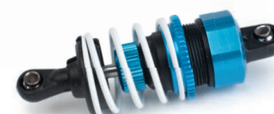
big bore oil-filled shock incorporate threaded bodies for easy ride height adjustment
