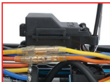
Bullet connectors are used between the speed control and motor
