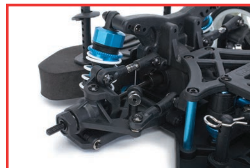
Front and rear anti-roll bars are a nice feature, hinting at the S10 Blast TC 2's race potential
