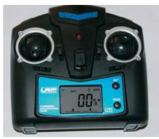
The basic 2.4 GHz FHSS transmitter has digital trims plus two additional function buttons (mode select and 360 deg flip) on the front panel; the LED display here shows zero throttle, selected switch state and battery level
