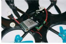
The small LiPo slides into the battery cradle mounted underneath
