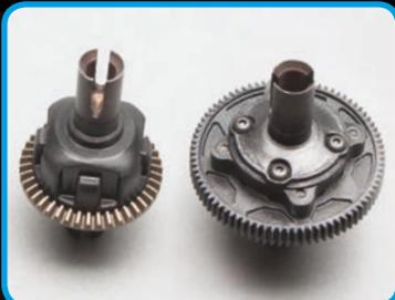
New gear differentials have machined steel ring, pinion, and planetary gears
