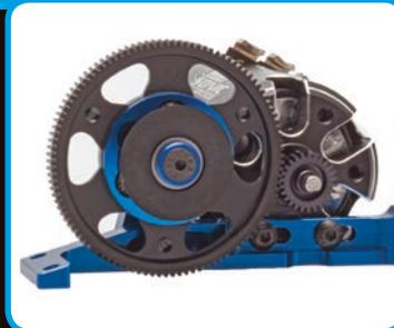
*New one-piece motor mount with central mounting to allow free chassis flex in either direction*
